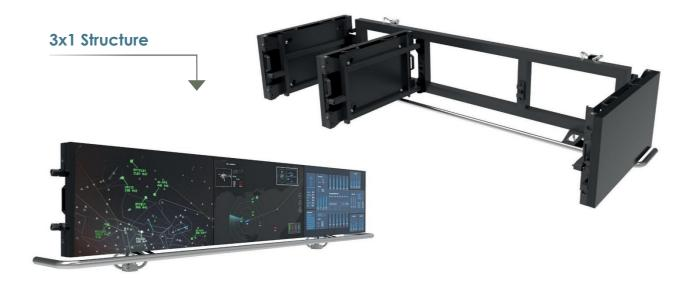
The Irts's patented structure is qualified to resist shock and vibration inputs up to MIL S 901D Grade B, and sustains up to 1 grms in vibrations from 10 to 100 Hz.. The folding and sliding shutter-system provides a quick installation and maintenance solution.
