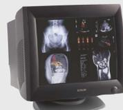
*Digital mammography requires high-resolution displays to show images with filmlike precision. This kind of resolution can only be obtained with **monochromatic (grayscale) monitors**.*
