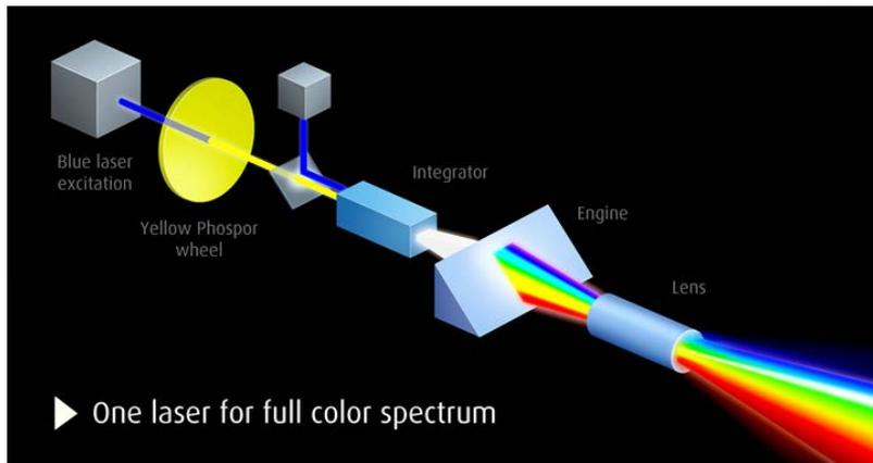
Fig.2 A high-level concept of a blue-pumped laser phosphor projector
