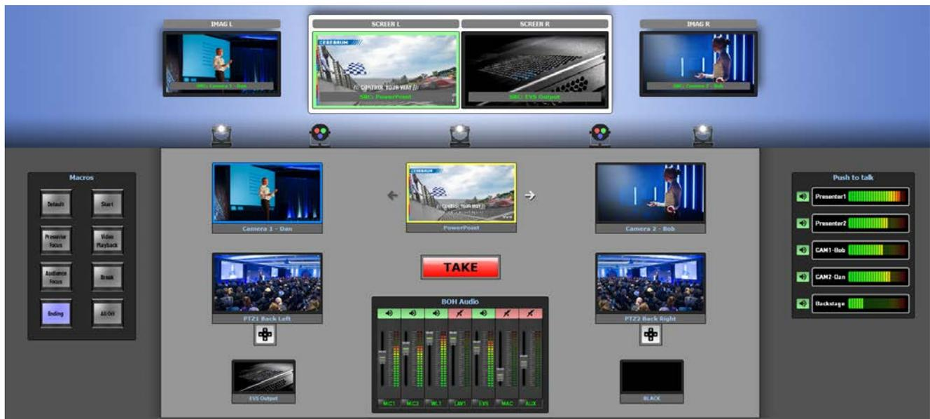
*Interface example: In this interface you can control the inputs and outputs of the E2 system (which screen should show which source) as well as controlling intercom, PTZ camera's, lighting equipment, audio mixers, presentations and launching salvos and macros.*
