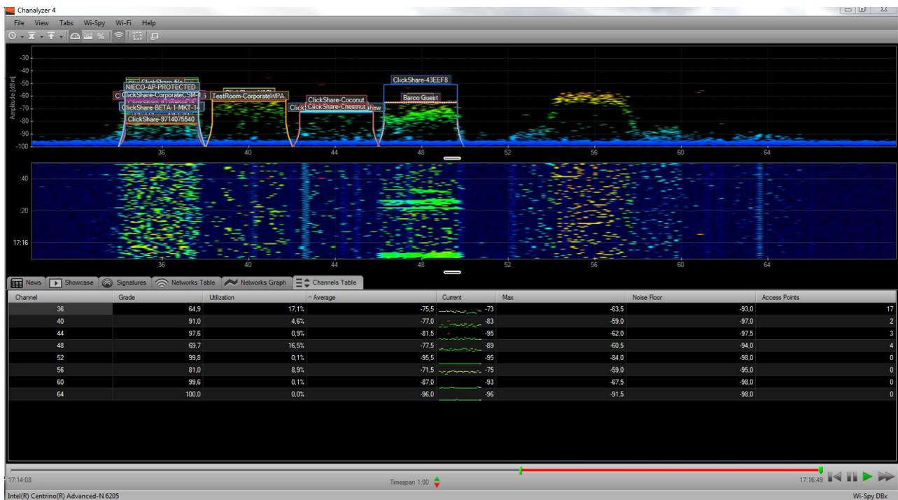
Figure 2: Screen capture of the InSSIDer spectrum survey tool (<http://www.inssider.com/>)
