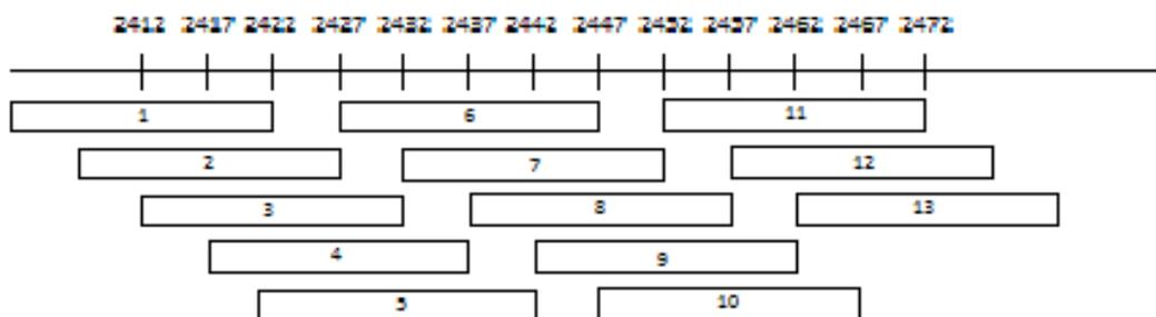
Figure 1: Wi-Fi channels in the 2.4GHz band
