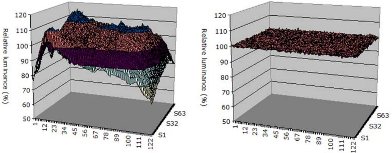
In addition to luminance variations, shown in the exaggerated gray image on the left below, there are color variations. As the display is made up of red, green, and blue sub-pixels, it happens that one area of the screen will have a different color temperature than another area. Simply put, both luminance and color variations are errors, and will introduce noise into the display.
