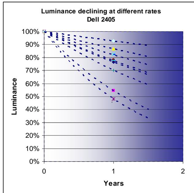
No radiologist would tolerate a situation where some seldom-used displays are still running at 80-90% of the original luminance while others are running at 40-50%. When using commercial displays for radiology there is an additional burden of frequently checking all the displays, retiring some, and adjusting others.
