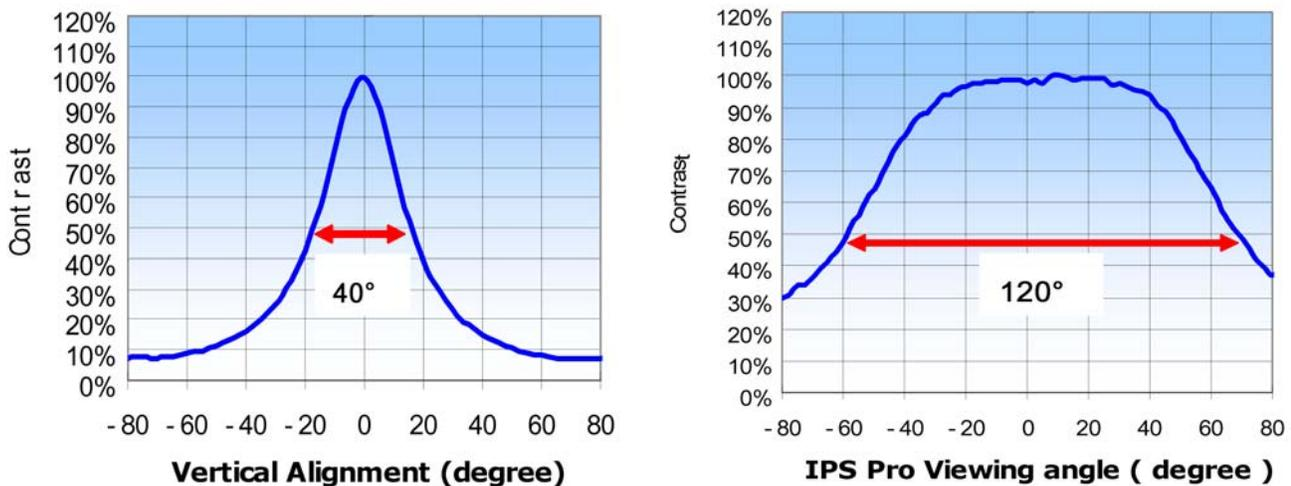
In fact, since 2007, commercial displays have increasingly switched toward an even-less appropriate LCD technique known as twisted nematic (TN). This technology is older and had been largely been discarded. Recently though, as cost pressures the commercial displays, they have started using it again.
